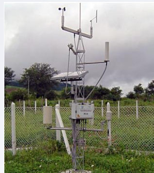
Picture 3. Automatic Data Collection Station (Brazilian Solar Energy Atlas, 2017).
